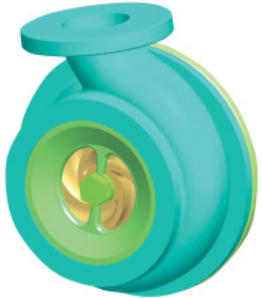
Geometry of a typical casing, impeller and cutter bar assembly
